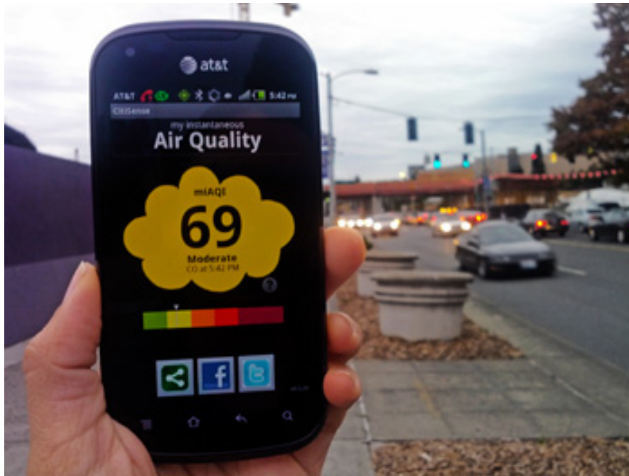
Figure 8: Prototyped “eco-phones” come equipped with air pollution sensors.
